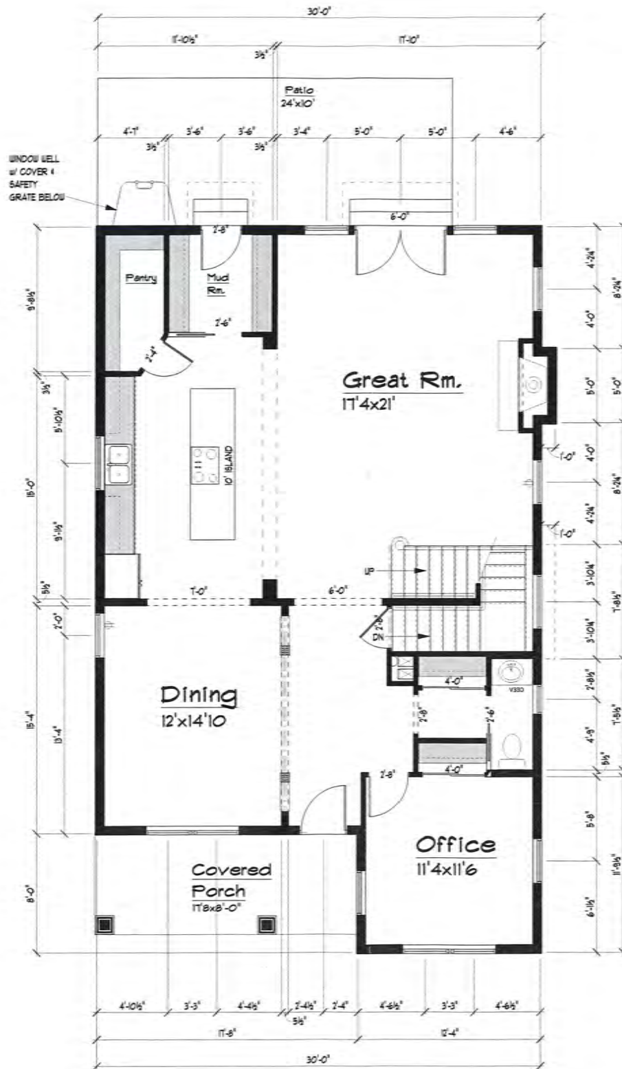
1st Floor Plan 1327sf. + 1328sf. 2nd Flr. = 2655sf. All room dimensions and square footages are approximate. Scale: 1/4"=1'-0"
