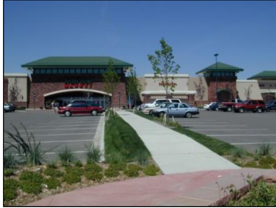
Figure 69-A: This photograph illustrates how a sidewalk connecting the public sidewalk to the business can be integrated into the required landscaping.
