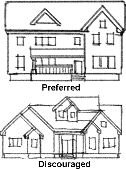
Figure 55-E: Illustrative example of preferred (top) and discourage (bottom) roof and eave lines
