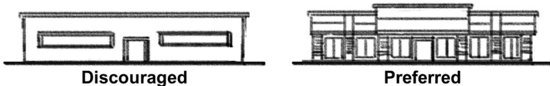
Figure 57-Q: Illustrative example of façade material variety
