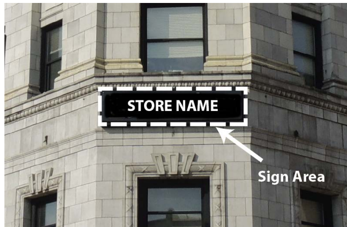
Figure 13-B: Illustration of computing the sign area for wall signs with a background panel or cabinet.
