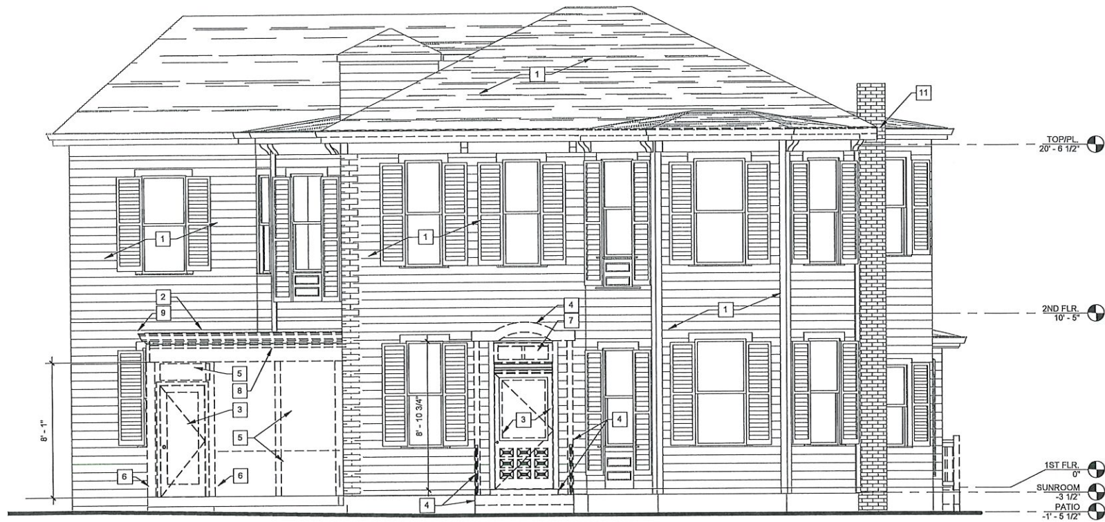
1 EXISTING / DEMO SOUTH ELEVATION A4 1/4" = 1'-0"
